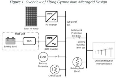
an AC-coupled system. A 30 kW three-phase Kohler gas generator is also interconnected to the microgrid system for supplemental power.
