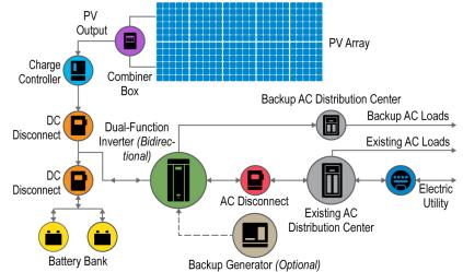
TYPICAL DC-COUPLED PV GRID-TIED SYSTEM WITH BATTERY BACKUP
