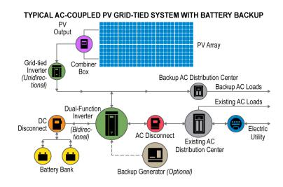
Figure 2. Typical components of a PV+ storage system (AC-coupled)
